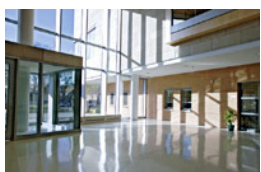
Bright Ideas Oversize windows and scuff-proof reflective floors made of recycled glass, plus a sensor system to reduce the need for artificial light, reduce the school's power use. Credit: JJ Sulin Photography
